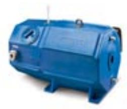
A unique combination of a conventional AC induction motor cooled with system hydraulic oil and hydraulic pump, either fixed vane pump or variable piston type, housed in a special sound reduction enclosure. This combination provides an exceptionally quiet and small pumping package for any industrial application requiring up to 125 horsepower (92 kilowatts) of continuous hydraulic power.
